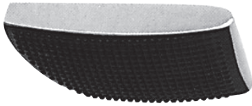
Toe Dolly, SPAENAUR No. 877-1045 - all polished, one face bowed and cross-milled for shrinking, length 120 mm, width 60 mm, height 28 mm, wt. 1,100 g.
